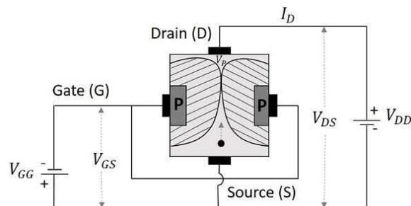
The voltage at which both these depletion layers literally “touch” is called as “**Pinch off voltage**”. It is indicated as  $V_P$ . The drain current is literally nil at this point. Hence the drain current is a function of reverse bias voltage at gate.
