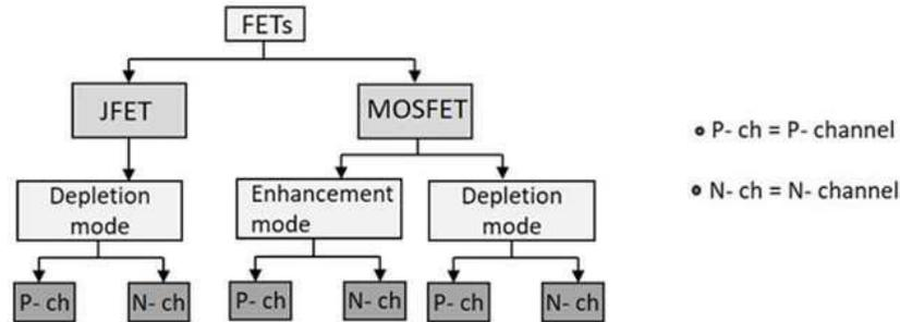
The JFET is abbreviated as **Junction Field Effect Transistor**. JFET is just like a normal FET. The types of JFET are n-channel FET and P-channel FET. A p-type material is added to the n-type substrate in n-channel FET, whereas an n-type material is added to the p-type substrate in p-channel FET.
