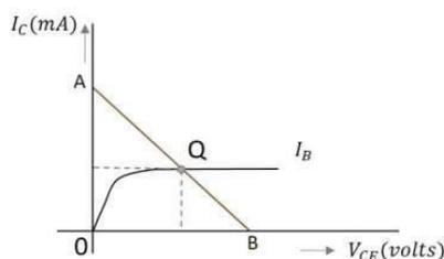
The load line has to be drawn in order to obtain the Q-point. A transistor acts as a good amplifier when it is in active region and when it is made to operate at Q-point, faithful amplification is achieved.
