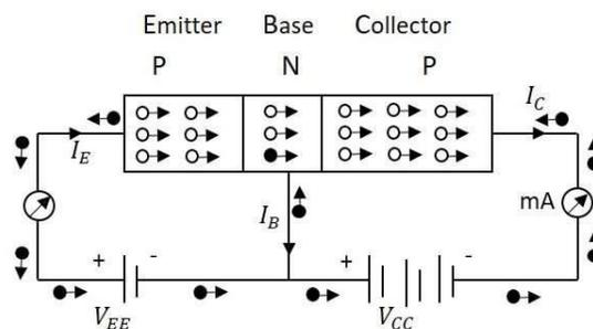
Operation of a PNP transistor
